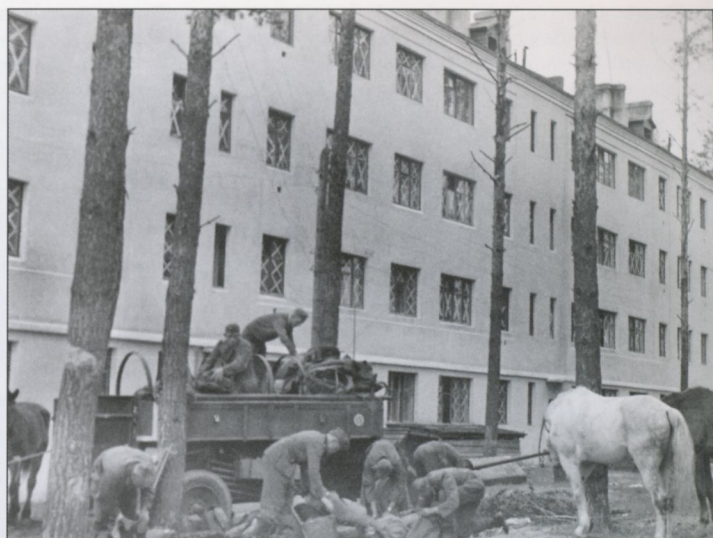
Only combat units were provided the modern Hf.7/11 large combat wagon (große Kampfwagen). It had a steel body and rubber ties. Behind the side panels were storage compartments. They were drawn by two horses and could carry 1.5 tons of cargo. The wagons were usually camouflage-painted on the exterior and the interior of the cargo bed was field gray. Note the paper stripes glued to the apartment block's windows.
