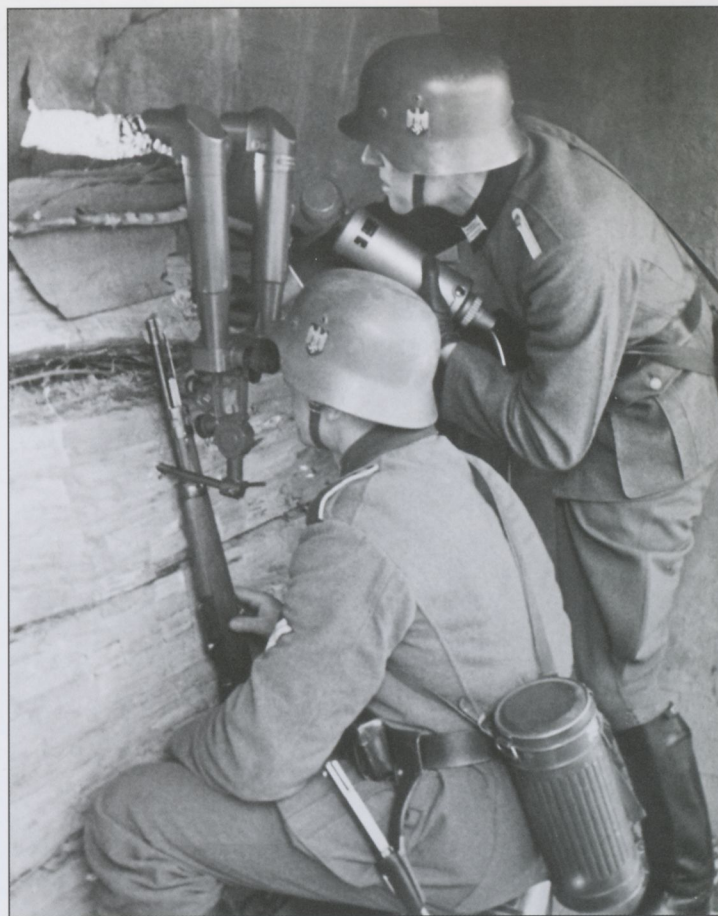
An Obergefreiter in a lookout post (Feldwachstelle) peers through a 6x30 Sf.14Z scissors binoculars (Scherenfernrohr), known as Eselsohren (donkey ears) for obvious reasons. Normally mounted on a high tripod, it was supplied with a spike to drive into wood or masonry for mounting in difficult positions. The Leutnant next to him with a microphone is a war correspondent recording a frontline narrative.
