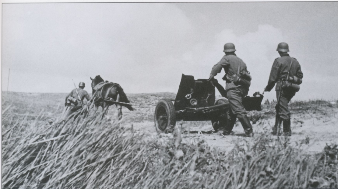
The crew of a 3.7cm PaK35/36 antitank gun gets an assist. Rather than manhandling the 970-pound (440-kilogram) gun to its position by themselves they have hitched a horse to the gun and lift the trails off the ground as the horse is led forward.
