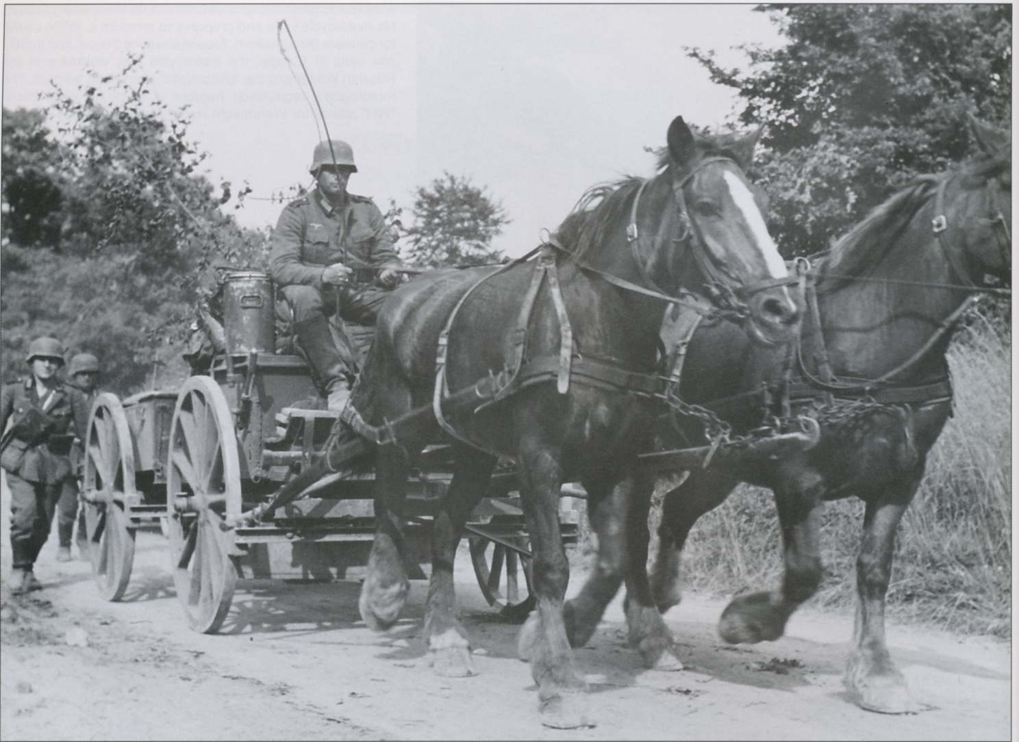
A small field kitchen (Feldküche) moves forward with the troops. The Landsers knew it as a goulash cannon (Gulaschkanone) or as a fodder cannon (Futterkanone) owing to its stovepipe, which is hidden behind the driver. On the driver's seat is an insulated ration container. One man could operate the field kitchen and it could continue to operate on their move. Every attempt was made to provide two hot meals a day.
